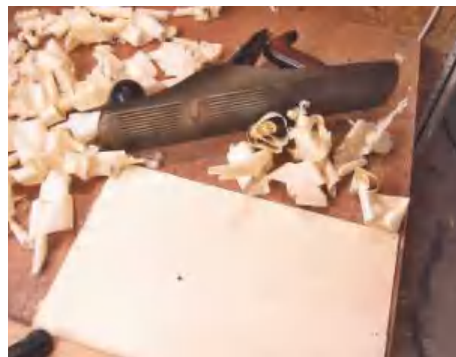
▲ Pic.33 The soundboard is reduced to 2mm thickness
